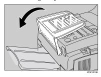
Push down on the paper until you hear the base plate lock into place.
