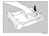
4 Prepare a stack of blank paper. For smoother operation, square the edges by tapping the paper stack on the bench.
