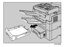
2 Lift the document delivery table and remove any jammed paper from inside the machine.
