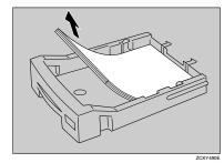
**U** If the metal base plate is raised, push it firmly down until it locks into place.
